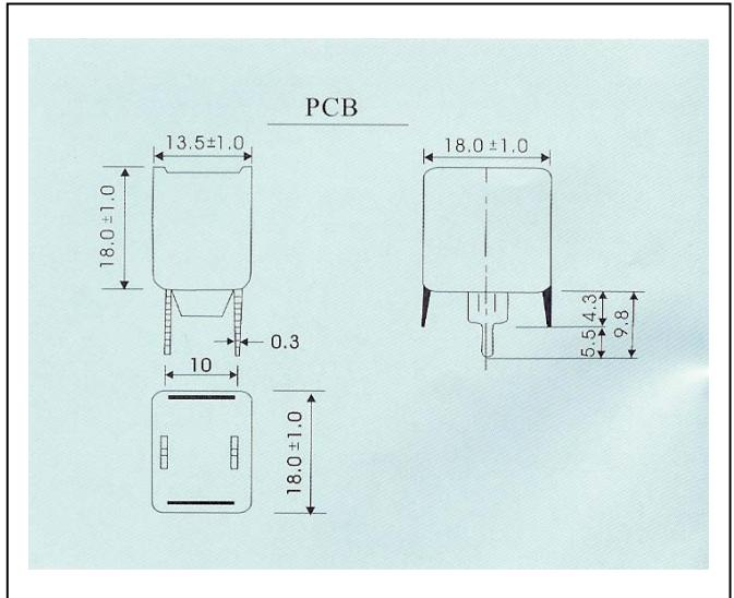
Degaussing PTC Thermistors are specially designed for applications in automatic degaussing circuits of color TV's and monitors etc. Degaussing Circuits Thermistors with low residual current provide quick response and rapid recovery for large inrush current and applicable practically to all power supplies. The Phenolic-base housings are self-extinguishing fire retardant conform to Bulletin 94V-0 of UL Standards.
